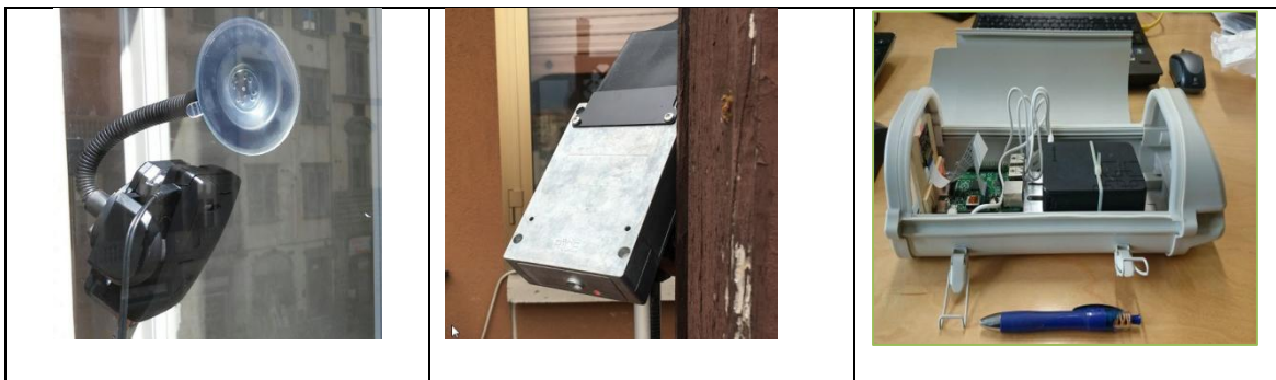
Three main variants of Traffic Flow sensors developed so far: Indoor with behind-window support (left), outdoor with waterproof case (center), autonomous station with battery (right).
