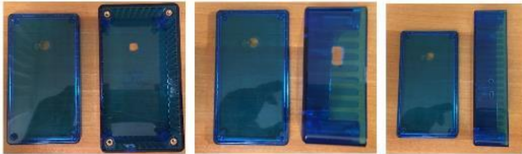
Figure 6 – YouSense devices box adapted to the PCB (Mini - Fixed)
