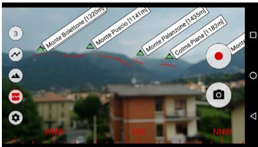
Figure 15: real-time skyline extraction peak identification and alignment, after strong tilt of the phone
